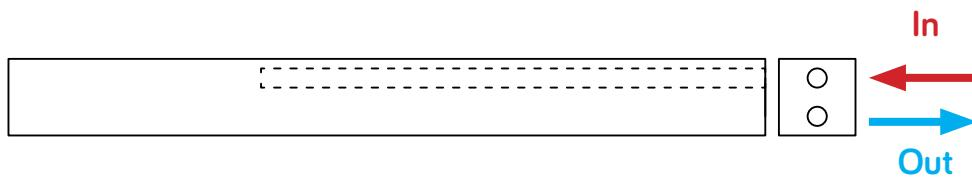
Our radiators are tested in qualified laboratories according to EN-442 regulations which determine the output value by fixing the  $\Delta T$  at 50 °C.  $\Delta T$  is the difference between the average temperature of the water inside the radiator and the room temperature. The formula is:  $((T_1+T_2)/2)-T_3$ .
